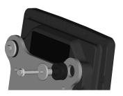
If the supplied isolator plate is not used, another plate or bracket with 5mm thickness can be used. The mounting holes are 16mm diameter on a 120x150mm rectangular pattern. Please provide clearance for the buttons on the side and the cables on the bottom.
