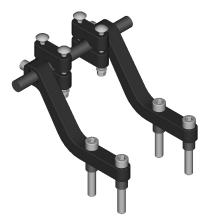
The mount arms accommodate handlbar clamps that use M8 bolts on 38-40mm spacing. The bolt length should be checked for proper thread engagement in the bar clamp.
